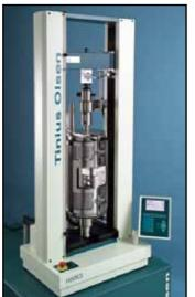
by a PC and software, whereas the S series has a built in display which allows quick simple tests to be performed, in addition to being able to be controlled from a PC and software.
