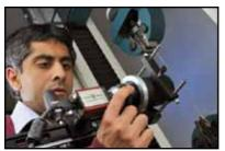
testing is being being used, Tinius Olsen has a couple of solutions to offer. The first one is a laser extensometer and the other is a video extensometer; both are non-contact methods and suited to a wide range of temperature limits and can still maintain extremely high accuracy.
